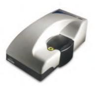
The Zetasizer Nano ZS90 offers the highest ever sensitivity, accuracy and resolution for the measurement of zeta potential of particles and surfaces. This is achieved by a combination of laser Doppler velocimetry and phase analysis light scattering (PALS) in Malvern's patented M3-PALS technique. Even samples of very low mobility can be analysed and their mobility distributions calculated.
